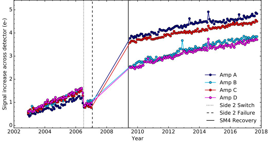
**Figure 2:** Same as Figure 1, but for observed ambient signal increase across the detector due to readout dark, in e<sup>-</sup>, over the lifetime of ACS. The signal increase was measured from raw bias images as described in the text.
