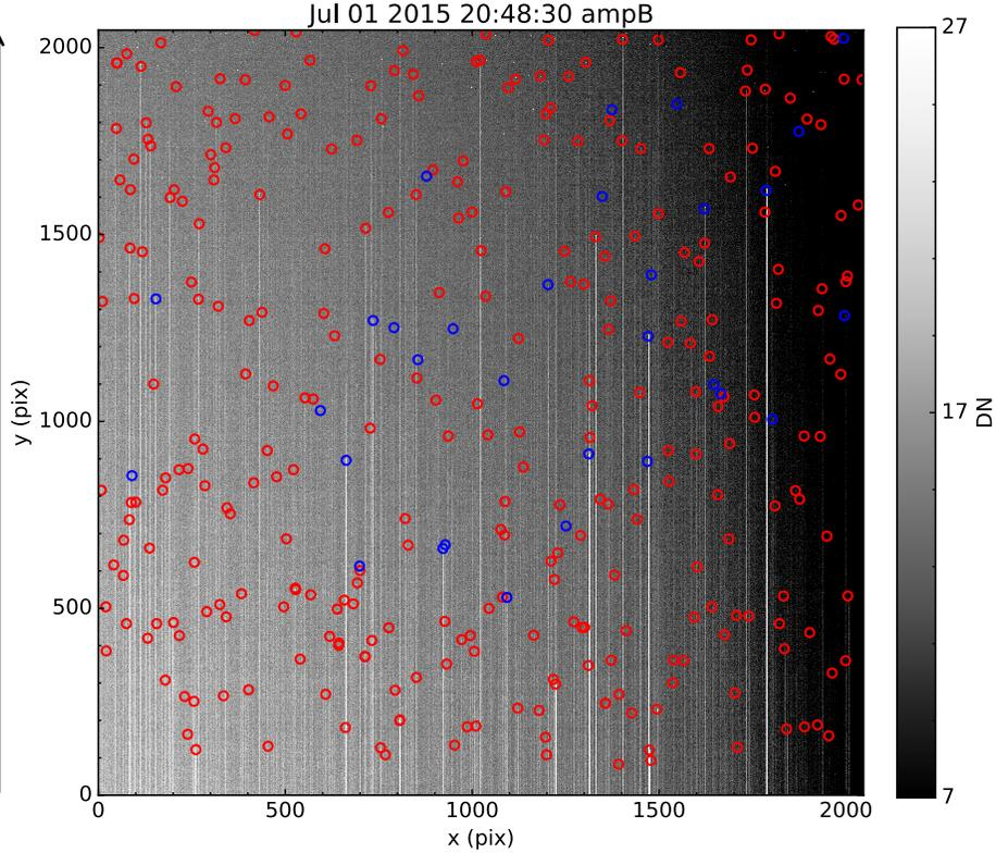
**Figure 8:** Top right quadrant (amp B) of the superbias from the 2015-07-01 anneal cycle. Hot columns are clearly visible as bright columns extending upward from the bottom of the frame. The circles mark the starting point of each hot column, with the red and blue circles representing stable and unstable columns, respectively, as discussed in Section 3.3. The black arrow on the left side represents the readout direction.
