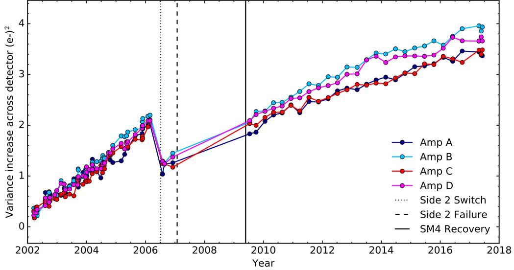
**Figure 3:** Same as Figure 1, but for simulated variance increase across the detector, in electrons squared,  $(e-)^2$ , due to readout dark as measured from simulated readout dark images over the lifetime of ACS.
