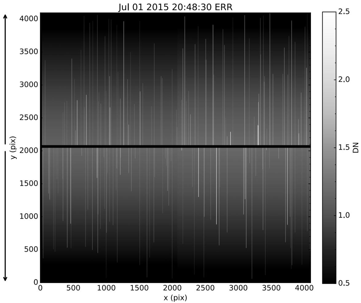
**Figure 11:** ERR extension, including contribution from the readout dark, of the superbias from the 2015-07-01 anneal cycle in units of DN. Both the ambient contribution to the noise and stable hot columns are clearly visible. The black arrows represent the readout directions for each chip.
