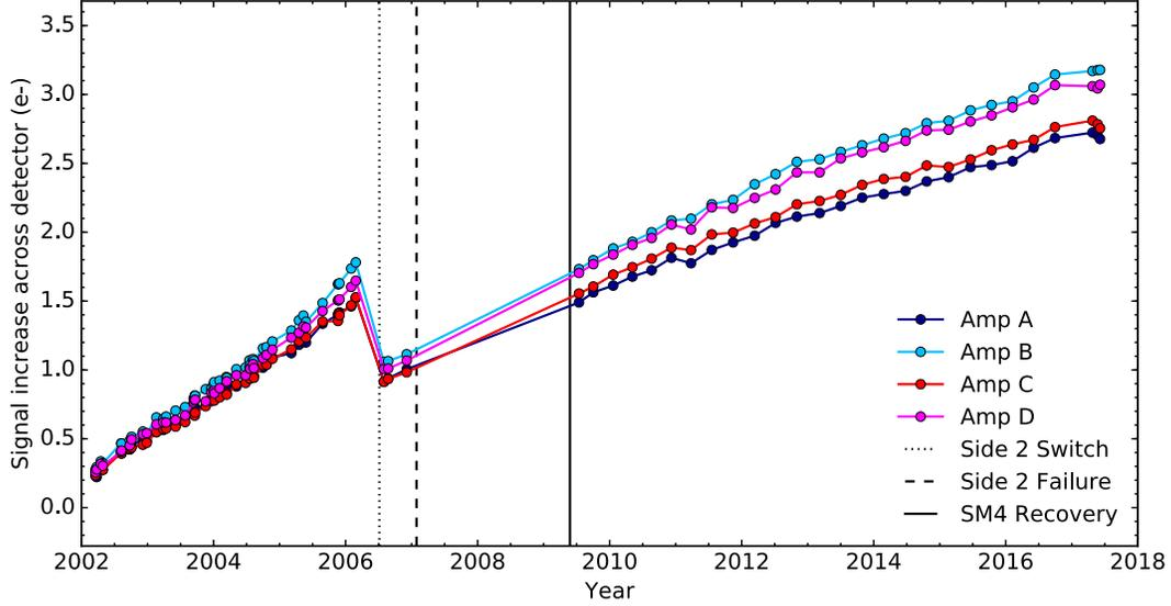
**Figure 1:** Simulated ambient signal increase across the detector due to readout dark, in  $e^-$ , over the lifetime of ACS. The signal increase was measured from simulated readout dark images as described in Procedure I. Each quadrant is labeled by the amplifier designation. The dates of the switch to side 2 electronics, the failure of side 2 electronics, and the SM4 recovery of ACS/WFC are also indicated by dotted, dashed, and solid black lines, respectively.
