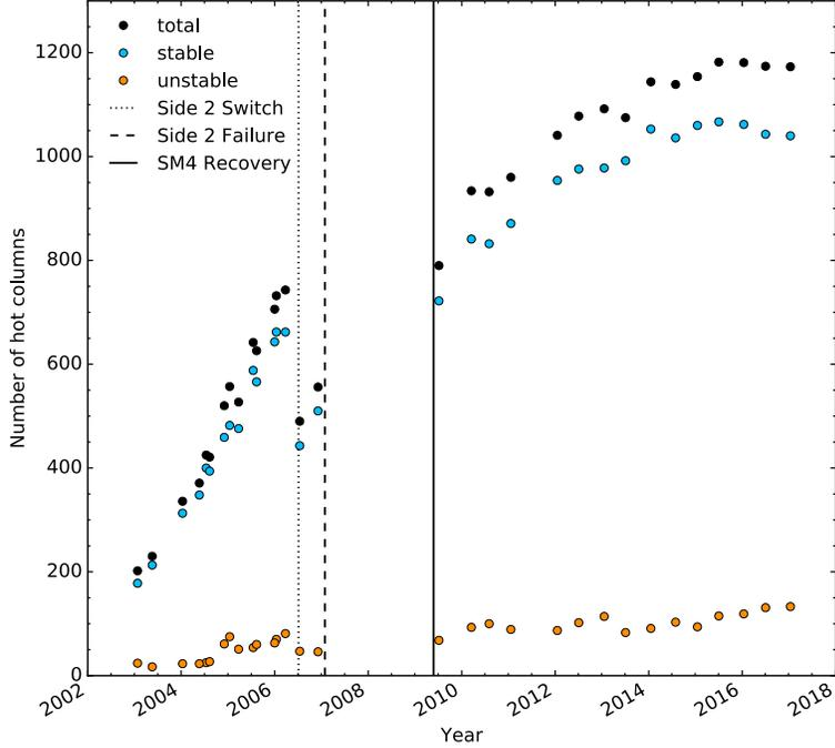
**Figure 10:** Number of hot columns identified in superbias using the methods described in Sections 3.2 and 3.3 as a function of time since ACS was installed. The black, blue, and orange points are the total, number of stable, and number of unstable hot columns, respectively. The dates of the switch to side 2 electronics, the failure of side 2 electronics, and the SM4 recovery of ACS/WFC are also indicated by the dotted, dashed, and solid black lines, respectively.
