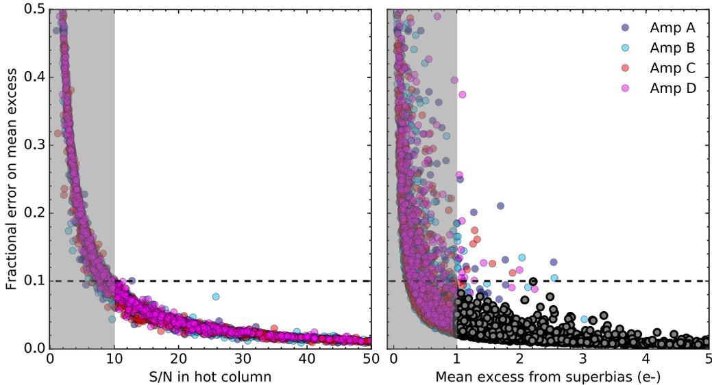
**Figure 7:** Fractional error of the mean excess in the hot columns as a function of  $S/N$  mean excess as measured in the superbias. Hot columns in each quadrant are color-coded. The gray shaded area covers rejected columns below the mean excess and  $S/N$  thresholds of 1 e $^-$  and 10, respectively. The dashed line represents a fractional error of 0.1 (10%). The gray points in the right panel are hot columns that satisfy both the mean excess and  $S/N$  thresholds.
