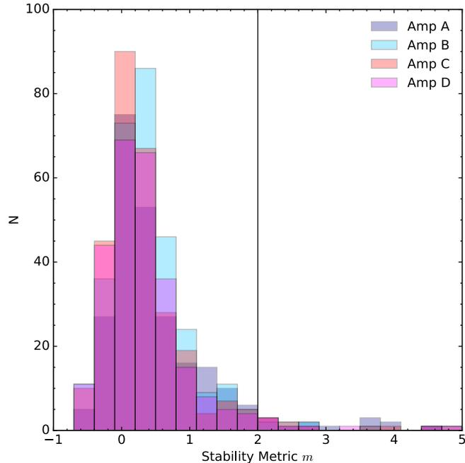
**Figure 9:** Distributions of stability metric  $m$  for hot columns selected from the 2015-07-01 superbias. Each quadrant’s histogram is color-coded. The vertical black line represents the threshold in stability metric that we use to differentiate between stable ( $m < 2$ ) and unstable ( $m > 2$ ) hot columns.
