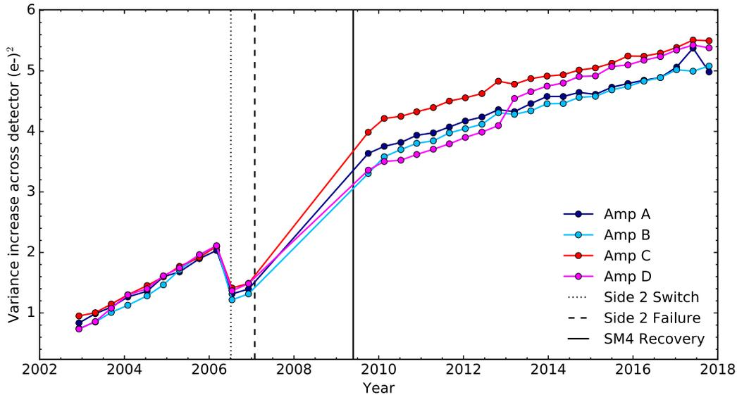
**Figure 4:** Same as Figure 1, but for observed variance increase across the detector in  $(e^-)^2$ , due to readout dark as measured from raw biases over the lifetime of ACS.
