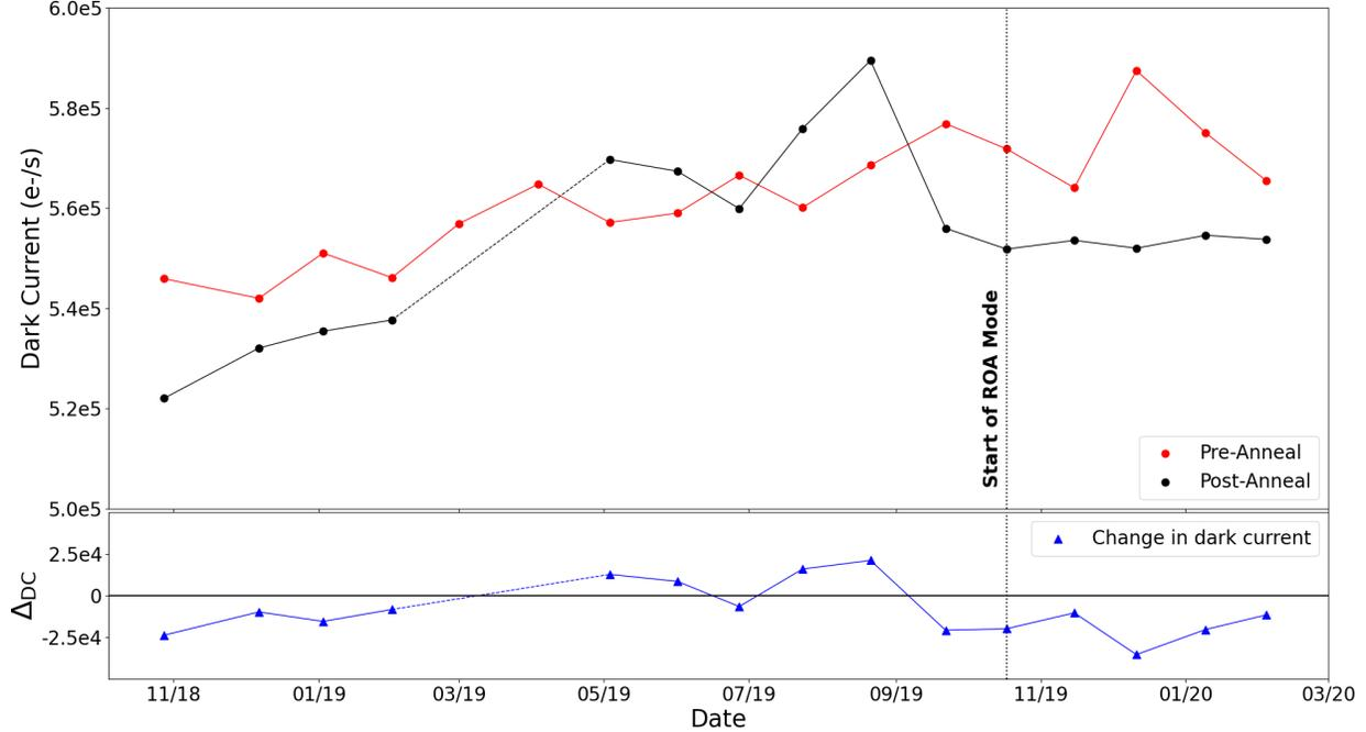
**Figure 1:** The global dark current pre- and post-anneal are measured alongside the change in global dark current ( $\Delta_{DC}$ ) with respect to each anneal. Each data point represents a set of calibrated and combined set of four darks from the CCD Hot Pixel Annealing program. The vertical dotted line indicates the start of ROA mode, while dashed lines connecting data points represent where data is missing.
