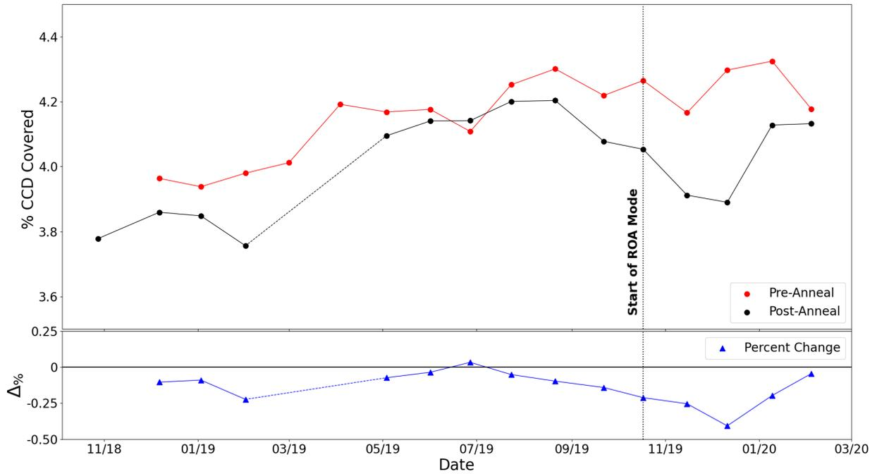
**Figure 3:** The percent CCD coverage of hot plus warm pixels pre- and post-anneal are measured alongside the change in percent coverage ( $\Delta\%$ ) with respect to each anneal. Each data point represents a set of calibrated and combined set of four darks from the Daily Monitor program. All line features are the same as described in Figure 1.
