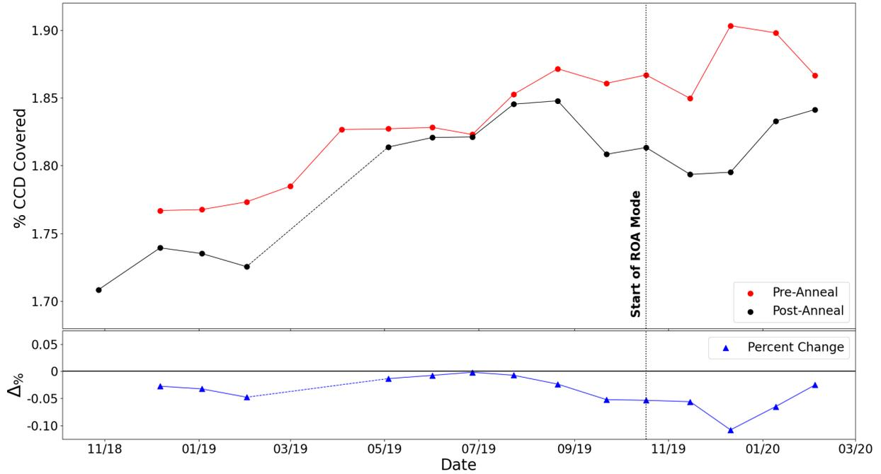
**Figure 2:** The percent CCD coverage of hot pixels pre- and post-anneal are measured alongside the change in percent coverage ( $\Delta\%$ ) with respect to each anneal. Each data point represents a set of calibrated and combined set of four darks from the Daily Monitor program. All line features are the same as described in Figure 1.
