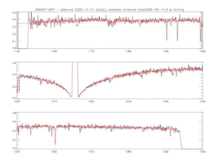
Example template is determined from SMOV high SNR program; observations were made in Sept. '09. Black curve is the raw spectrum, obtained in Dec. '09; red curve is the spectrum corrected with the template. Grid wires and some of the more egregious fixed pattern noise (at the edge of the detector) have been corrected.
