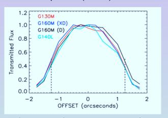
The left figure shows the relative COS aperture throughput as a function of XD or AD (D in figure) offset from the center of the aperture for all NUV gratings. The right figure is for the FUV.
