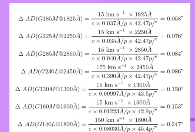
Assuming that the wavelength error budget is split evenly between the COS TA and wavelength scale accuracy, the allowable TA centering errors, in arcseconds("), are given in the table below. The strictest requirement for each grating is highlighted in RED.
