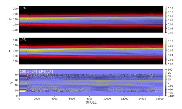
**Figure 3.** *Top:* The profile of G130/1291 FUVB at LP4. *Middle:* The profile of G130/1291 FUVB at LP3 for comparison with LP4. *Bottom:* The percent difference between the LP3 and LP4 profiles. The profiles at LP3 and LP4 are quite similar, and the differences between the two profiles reflect the slightly different optical path (field angle) and focus, which both affect the shape and width of the profiles.
