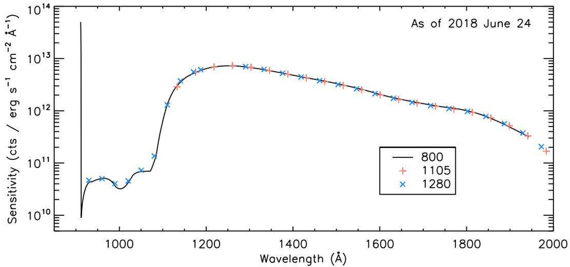
**Figure 1.** The G140L/800 sensitivity curve derived from spectra of WD0308–565. Note the  $y$ -axis is logarithmic. The large value at the shortest wavelength allows counts below 912 Å to remain in the final spectrum at artificially small fluxes pending a reliable calibration there. For comparison, the sensitivity curves for the other G140L modes, corrected to the time of the G140L/800 observations, are also shown at select wavelengths. They agree well with the result for cenwave 800.
