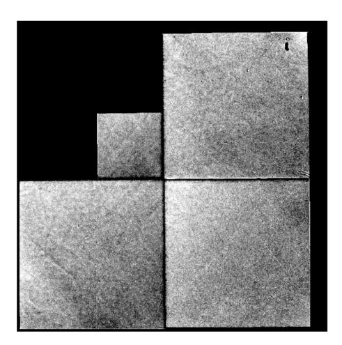
**Fig. 1.** Delta flat for F606W, i.e. the residuals for the epoch of the moon flats with respect to the current default pipeline flat field. The scaling is from 0.99 (black) to 1.01 (white). The CCD chips are numbered from 1 to 4 starting with the smaller PC field and counting counterclockwise.
