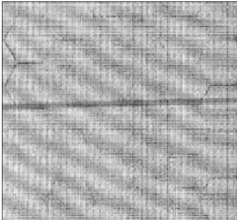
Figure 10: A portion of the preliminary FUV-MAMA high S/N flat. The tightly woven grid pattern is due to sensitivity variations between high-resolution pixels. These variations are due mostly to the way the MAMA detectors centroid the individual charge clouds, that is, counts are being re-distributed between adjacent pixels rather than being lost. These variations largely go away when the data is binned into the standard low resolution mode (1024x1024 pixel format) used by most observers. The hexagonal grid pattern is due to the way the fiber-optic cables are stacked in the MAMA manufacturing process. The wavy pattern is a beat pattern between the pores of the micro-channel plate and the anode array. The diagonal stripe is the shadow of the FUV-MAMA repeller wire, which is masked in the reference files. (Ferguson 1998)
