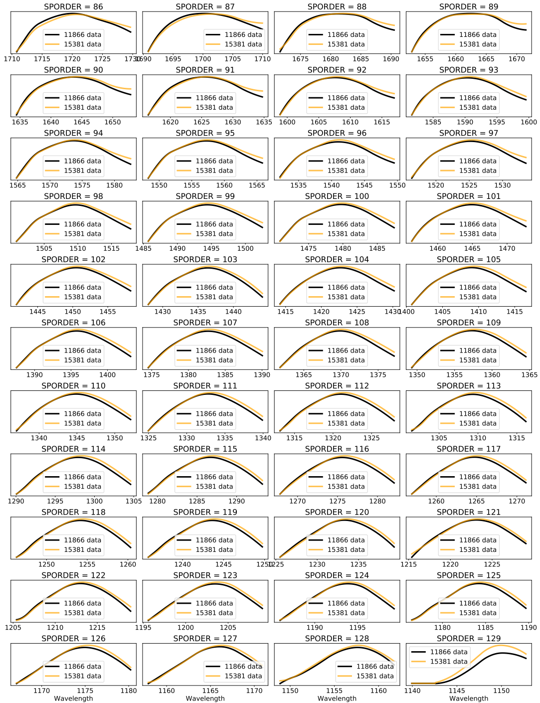
Figure 6. Comparison between the sensitivities of each echelle order as measured from the data taken as part of program 11866 and that taken as part of program 15381, using CALSPEC v07 models.
