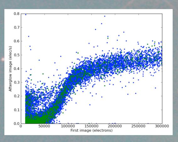
The plot to the left shows persistence signal rate as observed after a portion of the IR array was illuminated with a bright star. Note that the persistence is fairly small until the exposure level reaches about 2/3 of full well (50,000 e<sup>-</sup>). The plot at right shows the decay of persistence signal with time. Note that the nominal dark current rate is 0.04 e-/sec.
