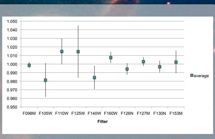
The error bars are +/- one standard deviation, which is between 1-2%, with the exception of F125W, photometry is affected by bad pixels in a couple of images.
