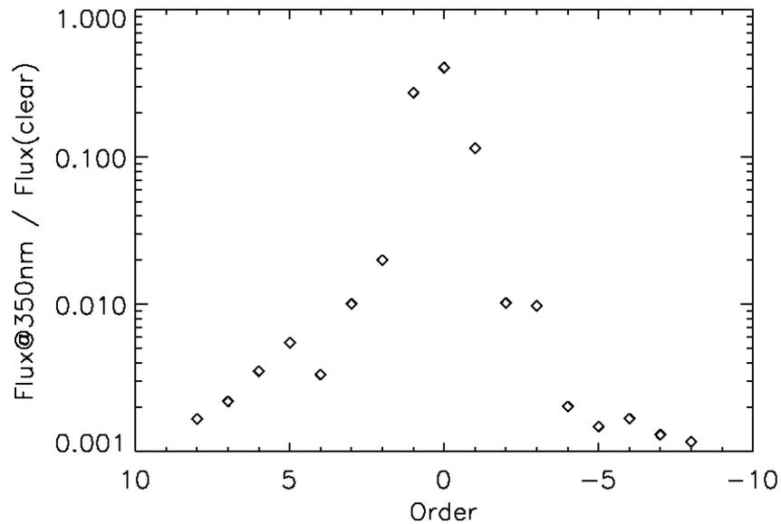
**Figure 7:** Measured flux in orders -8..+8 relative to a direct image is shown for a monochromator setting of 350 nm.
