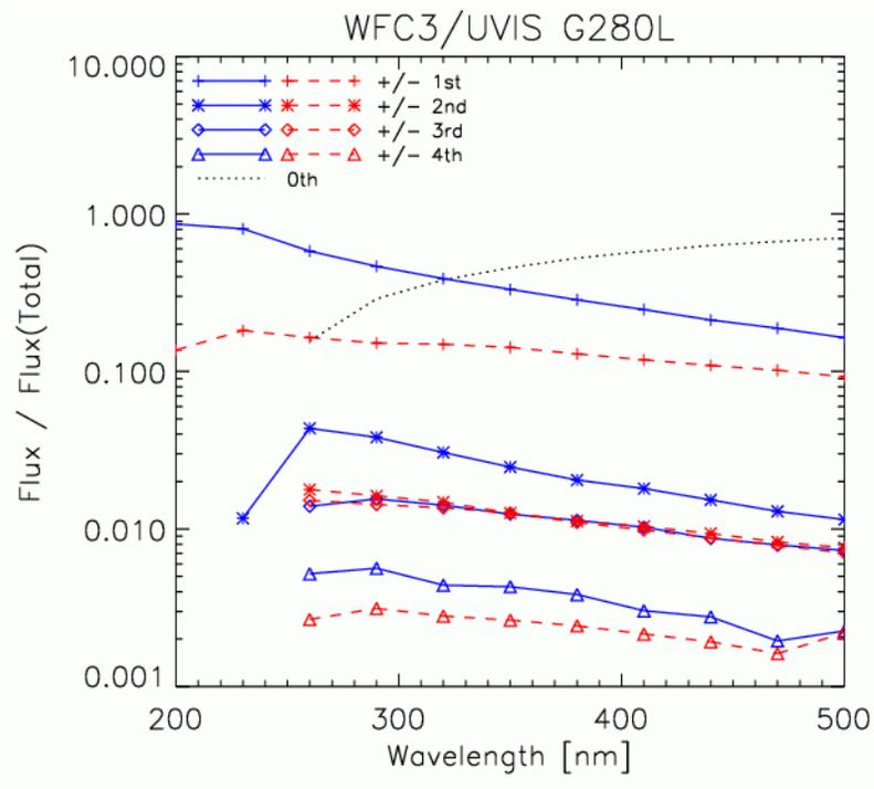
**Figure 6:** The flux measured in orders 0..+/-4, relative to the total flux in all orders, as a function of wavelength. Positive and negative orders are shown with solid blue and dashed red lines, respectively.
