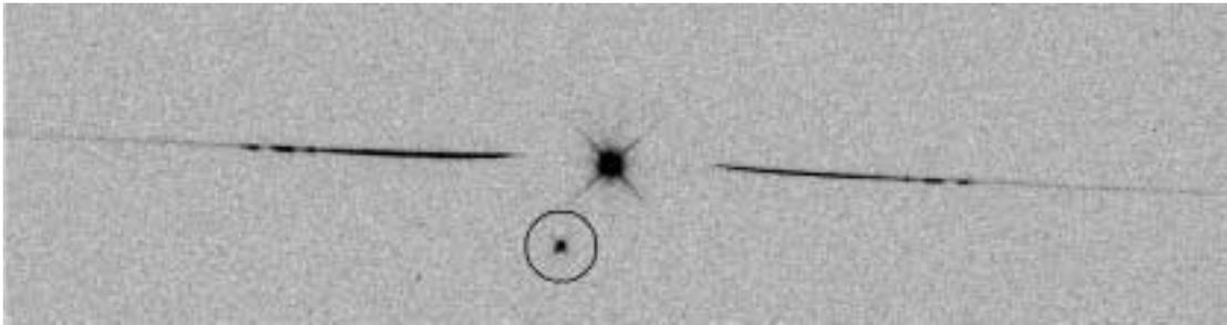
**Figure 1:** *Sum of a direct image taken through the F300W filter (marked with a circle) and the G280L spectrum of a continuum source. Note the dominating 0th order, the significant offset between the direct image and the spectra, and the curvature of the +/-1st order spectral traces near their blue end.*
