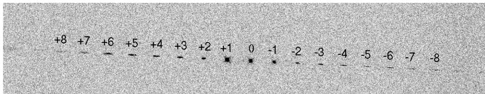
**Figure 4:** Section of a G280L exposure on Chip 1 for the 290 nm monochromator setting from the thermal vacuum test series. Orders from -8 to +8 are labeled.
