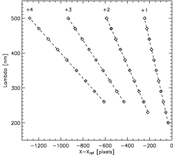
**Figure 5:** Wavelength solutions for orders +1 to +4. Note the overlap between the higher orders. Measured points are shown by circles and the fitted dispersion solutions, from Table 4, by dashed lines.
