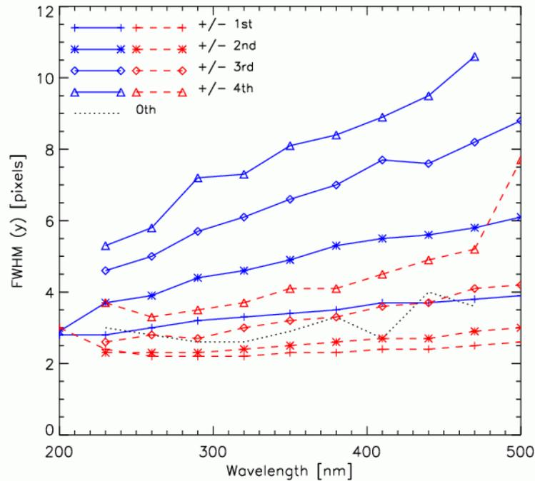
**Figure 8:** Full Width at Half Maximum measured along the  $y$ -direction for spectral orders -4..+4 is shown as a function of wavelength. Positive and negative orders are shown with solid blue and dashed red lines, respectively.
