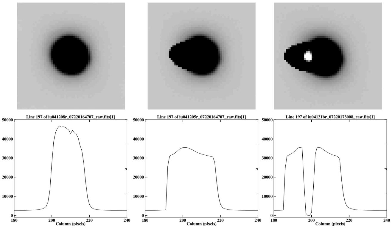
**Figure 2:** A 400x400 F555W subarray CASTLE flat read out through amp B (center) as compared to the corresponding 400x400 subsection of a four-amp readout F555W CASTLE flat (left). At right, quad B (2048x2051 pixels) from an over-exposed four-amp readout F410M calibration subsystem flatfield, illustrating the regions with zero pixels (white areas). Images displayed with an inverted color table and stretched to highlight features.
