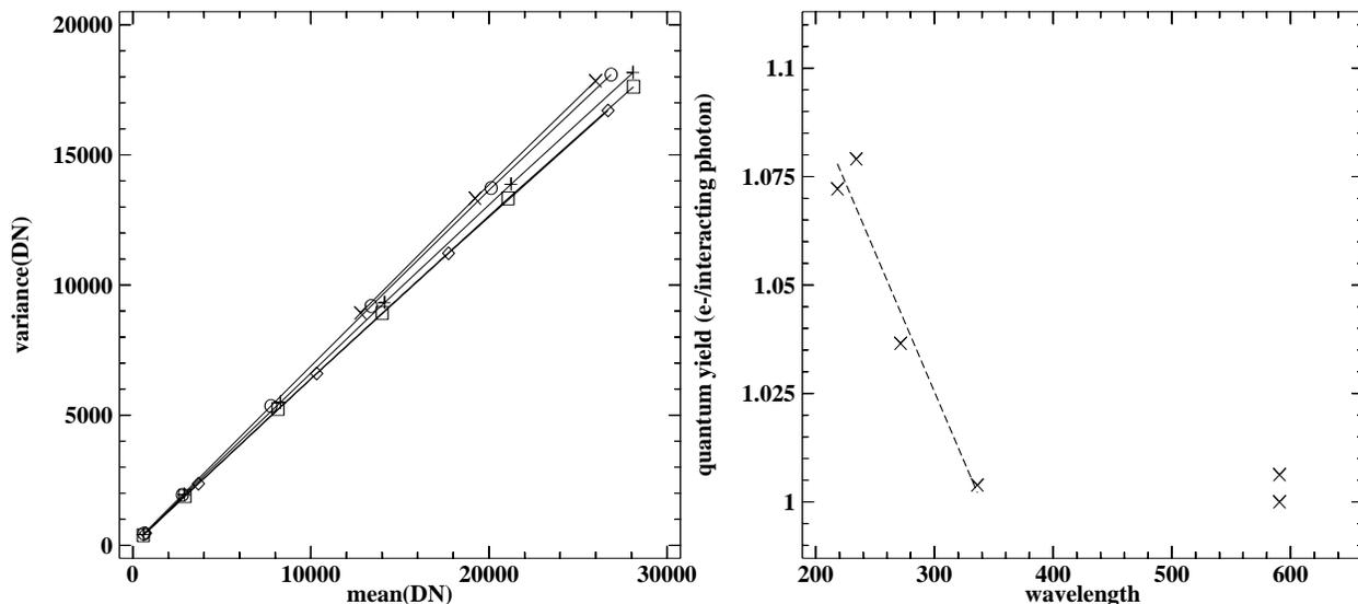
**Table 2.** Gain and quantum yield as a function of wavelength. Quantum yields are in units of  $e^-/\text{interacting photon}$ , with errors of  $\sim 0.02$  except for F218W, where they are  $\sim 0.06$ .
