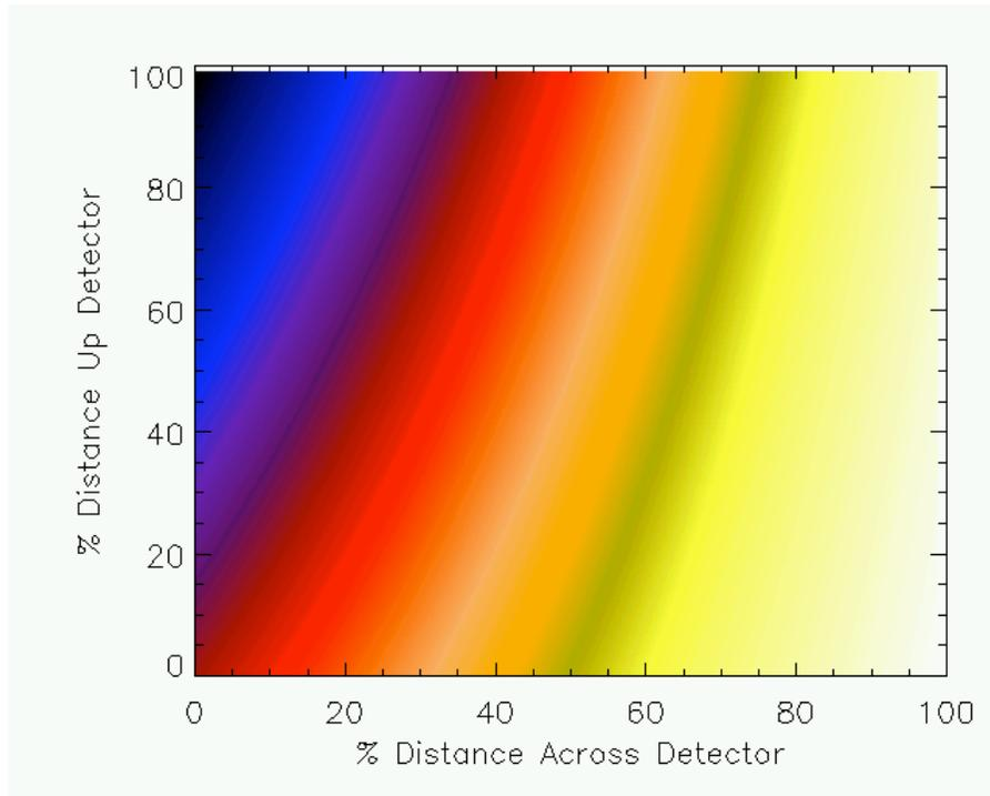
Figure 5: Contour plot of the fitted plane to the ratio image shown in Figure 4. The ratio values range from 36.062 in the upper left corner (amp A) to 36.125 in the lower right corner (amp D), in a direction slightly more horizontal than the detector diagonal. This implies a longer effective exposure time for the amp A corner relative to the amp D corner.
