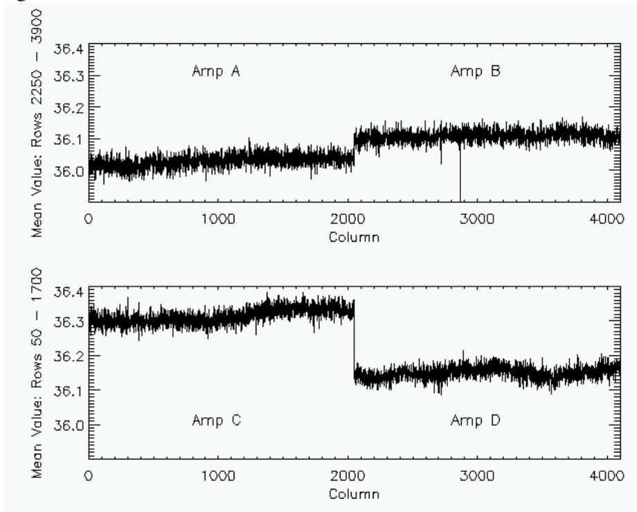
Figure 3: Plot of the signal in the ratio image along two mean rows. Each row was created by calculating the resistant mean across 1650 rows.
