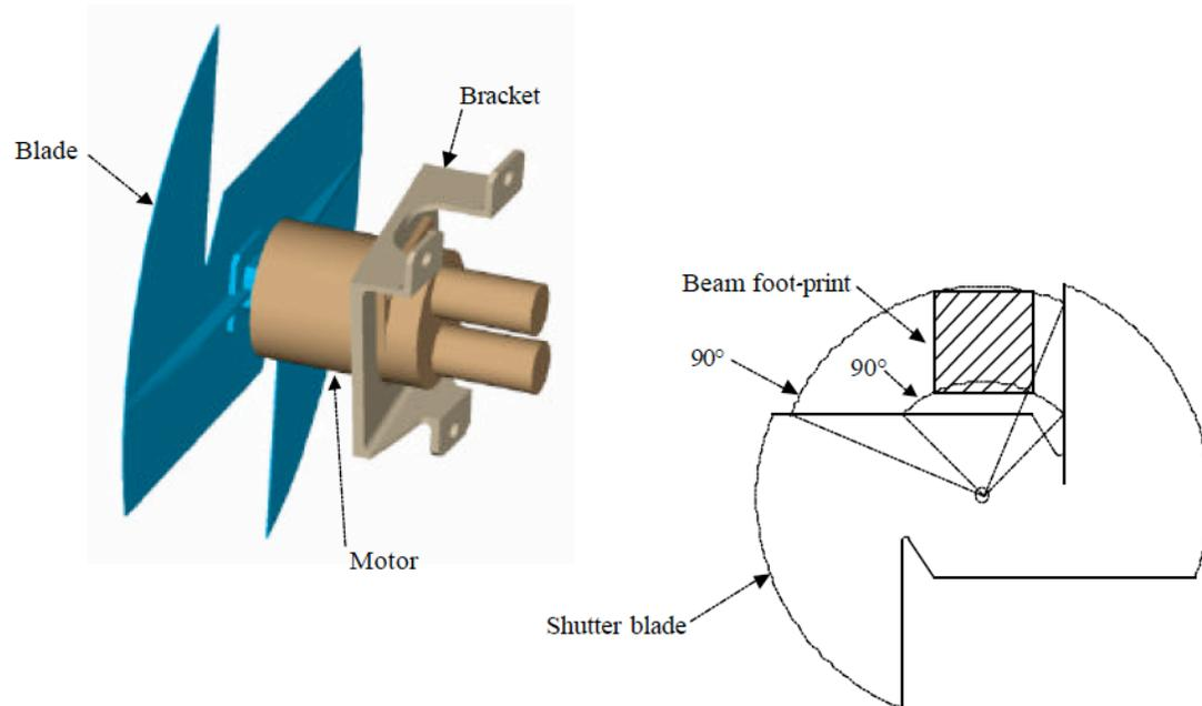
Figure 1: Graphical representation of the UVIS shutter mechanism, reproduced from the WFC3 OP-01 document (Baggett 2003).
