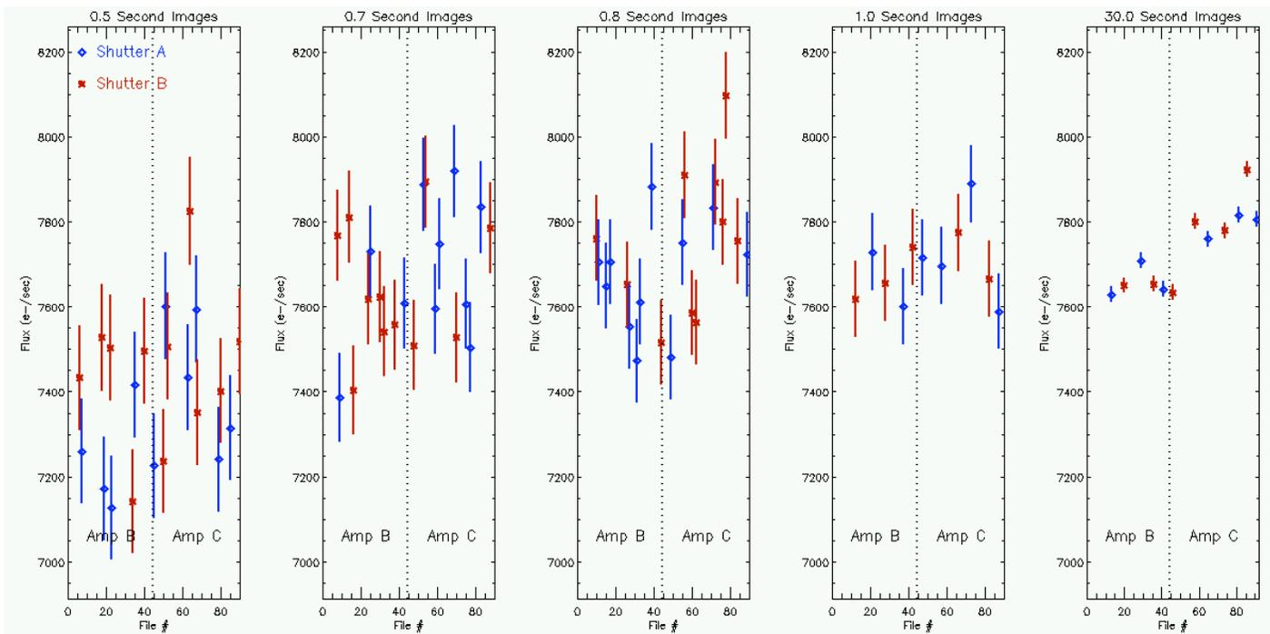
Figure 7: Measured countrates from each of the individual observations of GD153. Error bars are formal (Poisson) photometry error divided by commanded exposure time.
