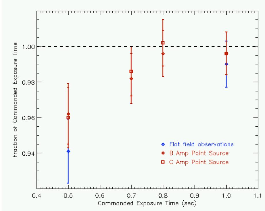
Figure 6: Shutter accuracy results derived from photometry on the mean image for each commanded exposure time presented in Table 4.
