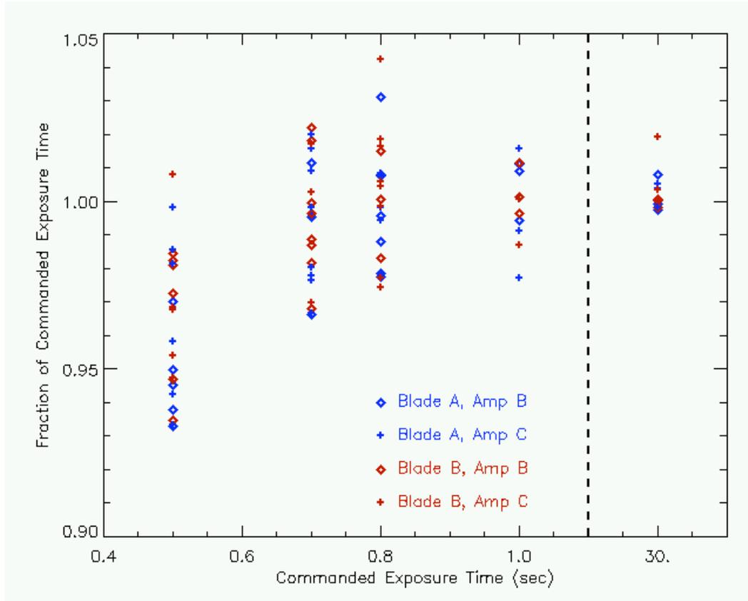
Figure 8: Countrate ratios calculated for each of the individual images of GD153, with distinctions made for each of the two shutter blades as well as the amplifier used.
