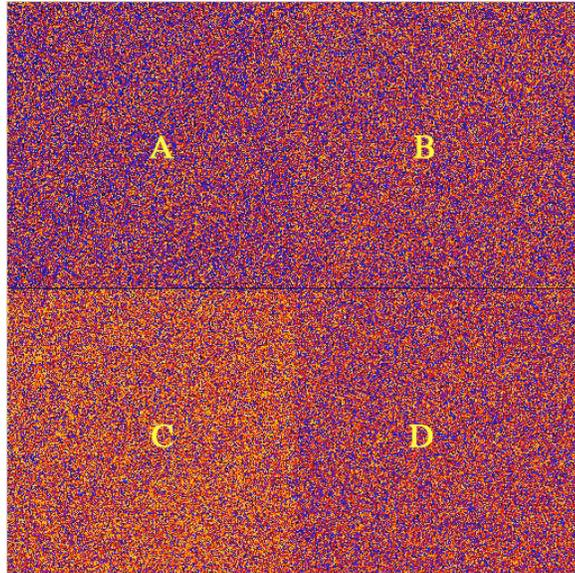
Figure 2: Ratio image of the mean 17.0 second flat to the mean 0.5 second flat, with the amplifier corresponding to each quadrant labeled. This is a histogram equalization stretch, ranging from 34 to 38.4. In this color scheme, blue represents the lowest values, with red, orange, and yellow representing successively higher values.
