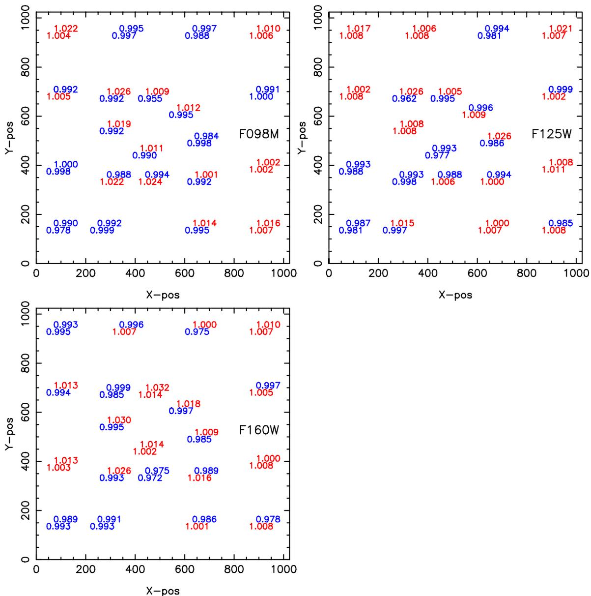
Fig. 2.— The flux as a function of position on the WFC3 IR detector derived from measurement of the standard star WD-1057+719 in three different filters, F098M (top left), F125W (top right), and F160W (bottom left). The flux is normalized by the mean flux in each filter, respectively. Values larger than one, in red, indicate that the measured photometry is brighter than the mean, while blue number indicates that the measured photometry is below the mean.
