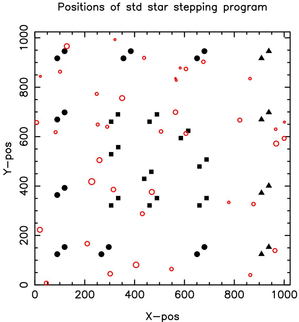
Fig. 1.— Black symbols show the positions of the standard star positions on the WFC3/IR detector. Different shapes indicate different exposure times (squares=4.3s, circles=8.8s, and triangles=22.9s). Red open circles indicate the positions and sizes of the IR blobs. We estimate that none of the measured standard star positions has photometry affected by the IR blobs.
