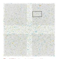
The MSA placed at this position on  $\Omega$ Cen can observe the stars marked +, while stars marked x are behind the inter-shutter bars or the few inoperable shutters. Observable stars in the same row will be covered by seperate configurations of the MSA.
