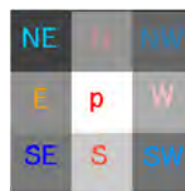
Figure 2. Central 9-pixel region used for analysis. Nine pixel types p (peak), E, W, N, S, NE, SE, SW and NW are marked.
