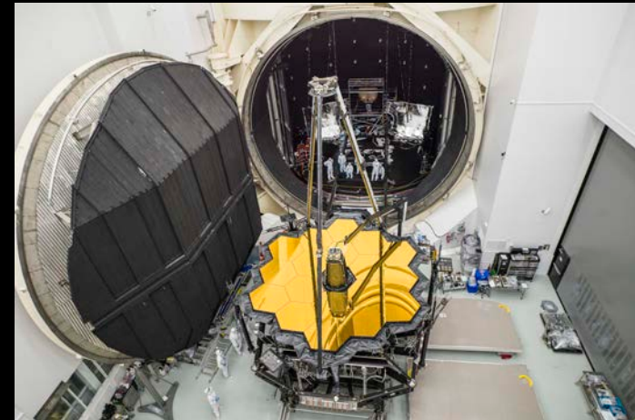
Telescope emerges after cryogenic testing at NASA/JSC
