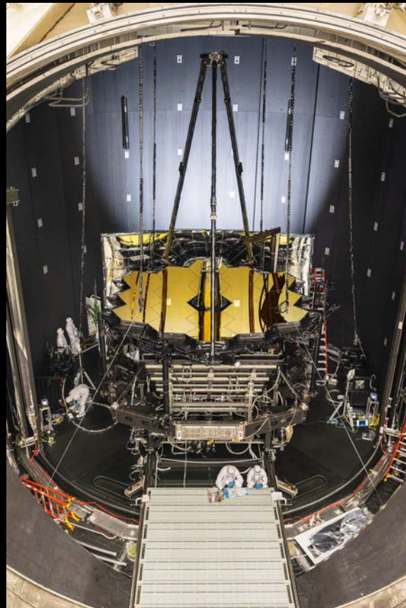
Webb Cryotesting at NASA Johnson Space Center
