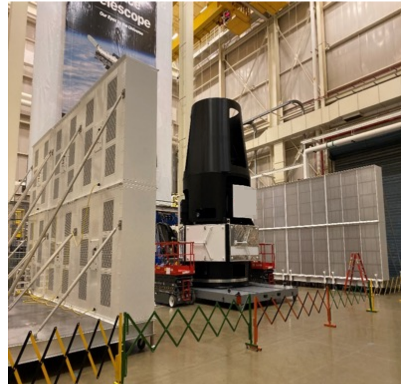
Six HEPA Dolly Push-Push Configuration using RST mock-up
