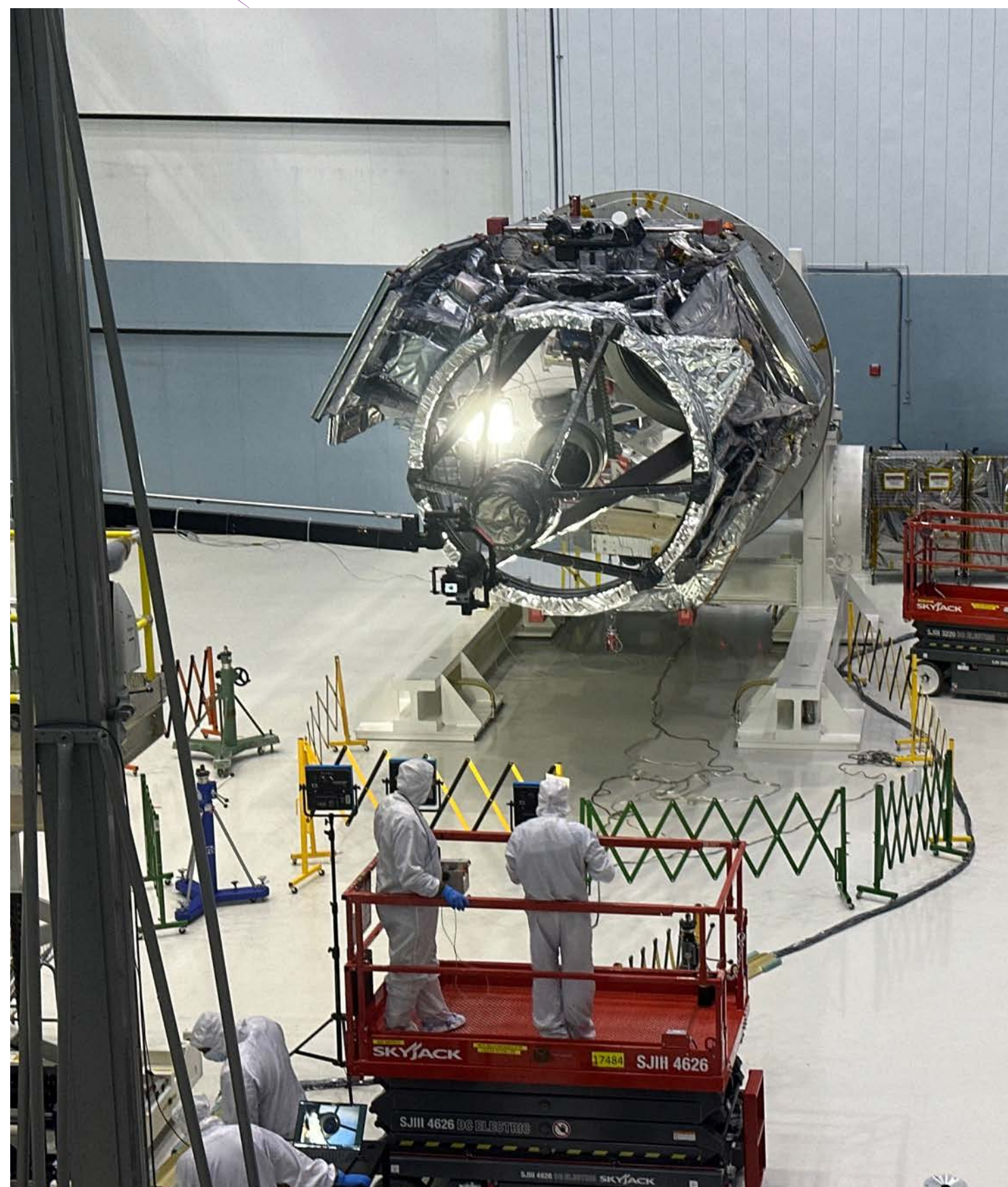
Thermal Vacuum Test (TVAC) of Spacecraft + Integrated Payload assembly (SCIPA) completed during shutdown in October; included end-to-end testing of data pipeline in coordination with STScI Roman Science Operation Center.
