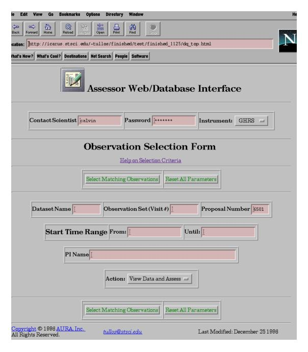
Enter a contact scientist username, password, instrument, and proceed to the **Observation Selection Form**, making using of any single selection criteria. The program fully supports any combination of individual selection criteria.
