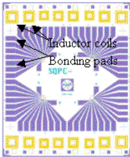
Figure 6. 8x10 mm substrate for SETs and submillimeter detectors. Chip has 16 rf tank circuits.
