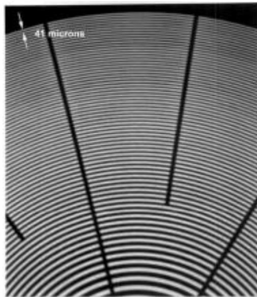
Figure 1. Picture of a 1-mm thick tungsten zone plate taken with 100 keV photons.
