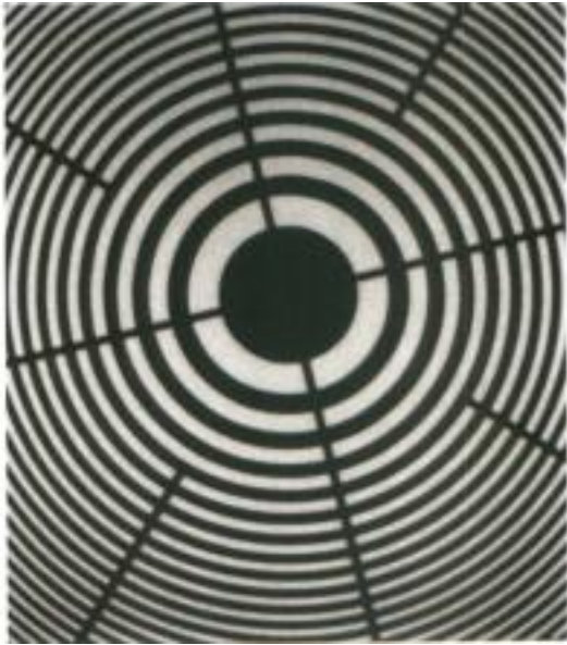
Figure 1. Picture of a 1-mm thick tungsten zone plate taken with 100 keV photons.
