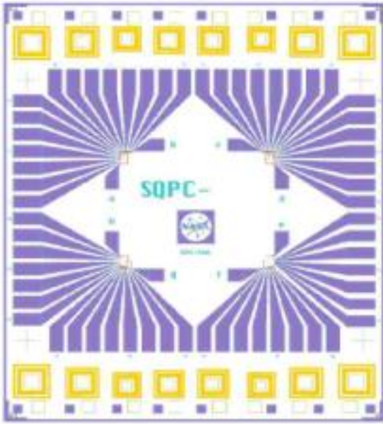
Figure 2: Layout of SQPC Chip (8 x 10 mm)
